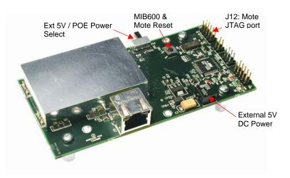
Figure 10-1. Photo of top side of an MIB600CA.
