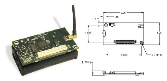
Figure 3-1. Photo of the MPR2400—MICAz with standard antenna.
