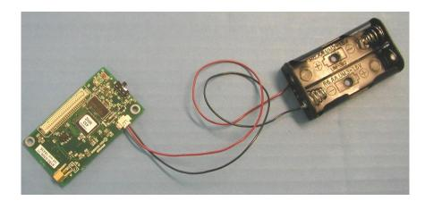
Figure 4-4. Photo of using the Molex connector to attach the AA battery pack. Photo courtesy of Nick Sitar, UC Berkeley, 2004.
