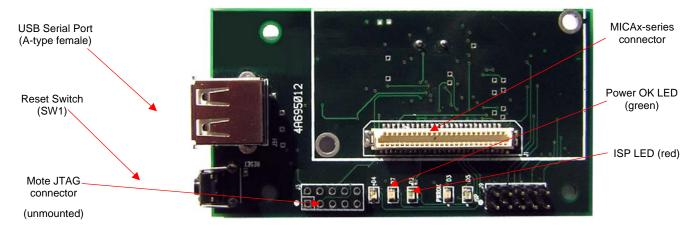
Figure 9-1a. Photo of top view of an MIB520CA.
