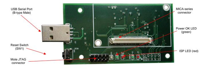
Figure 9-2b. Photo of top view of an MIB520CB.
