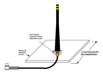
Figure 5-2. Illustration of an antenna option for the motes using a Linx antenna and ground plane.
