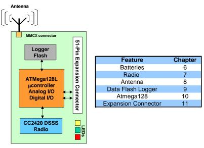
Figure 3-2. Block diagram of the MICAz and listing of Chapters that discuss the components in greater detail.
